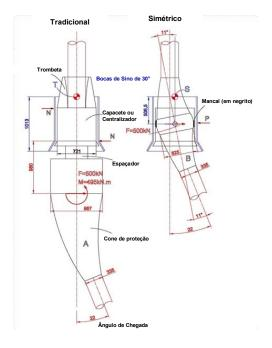
1) **Figure 1** above shows the diagram of two bending stiffeners: the one on the left represents a standard stiffener for a 9-inch riser with a 30-inch bell mouth (just shown); the one on the right shows the schematic of a zero bending moment stiffener, BSym, also for the same riser and the same 30-inch bell mouth. A summary study was designed to size the BSsim-concept so that both had the same performance under the action of extreme loading.
